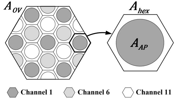
Fig. 2. An overlay network based on a regular hexagonal cell architecture
